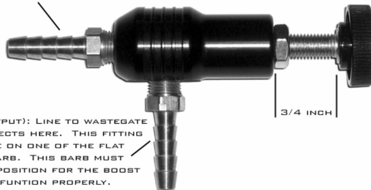
WASTEGATE (OUTPUT): LINE TO WASTEGATE ACTUATOR CONNECTS HERE. THIS FITTING HAS A TINY HOLE ON ONE OF THE FLAT SIDES OF THE BARB. THIS BARB MUST REMAIN IN THIS POSITION FOR THE BOOST CONTROLLER TO FUNCTION PROPERLY.
